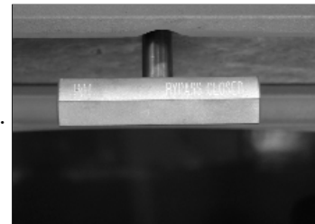
Use your bypass handle to engage or disengage your catalytic combustor. (Fig 1)
